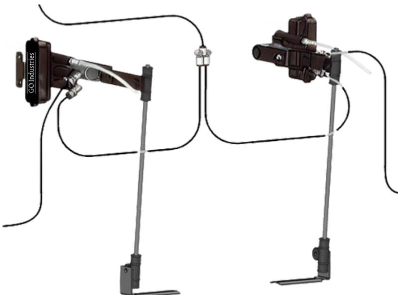
This adjustment relies on levelling valves (HCV) installed beneath the caravan that are connected to the suspension arm.
